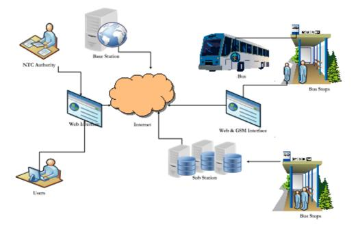
Fig. 4. Real time bus scheduling system model
