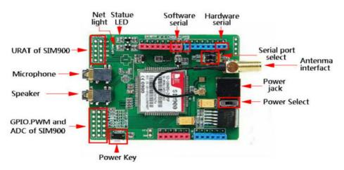
Fig. 3. Arduino GSM / GPRS Shield
